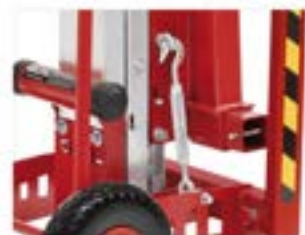
Adjustable mast blocking system for horizontal transportation.
